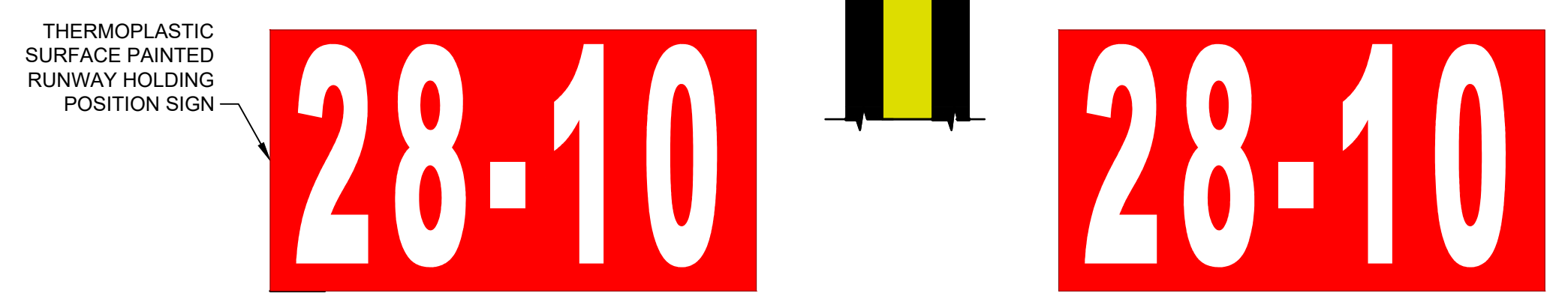
RUNWAY HOLDING POSITION MARKING 4 NTS MD-01
