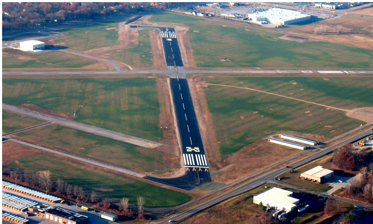
Figure 2-3. Markings for a Temporarily Closed Runway
